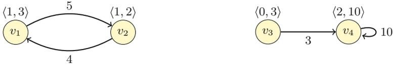
(a) A DRT task with two job types      (b) A periodic task with an initial phase of 3 modeled as a DRT task
