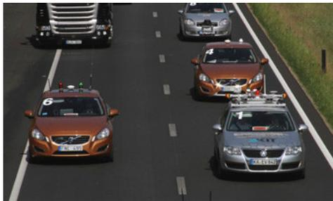
(c) Sensors can be used to provide information about the position of the cars in a challenge on cooperative and autonomous driving.
