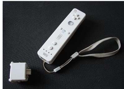
(c) A Wii controller containing an accelerometer and a Motion-Plus expansion device containing a gyroscope.<sup>2</sup>
