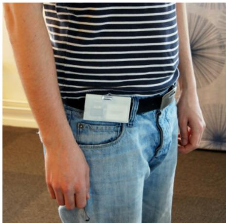
The sensors (IMU and radio) and the DSP are mounted inside an ID badge.
