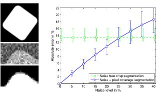
**Left:** (top) Synthetic test objects. (middle) Part of object with 30% noise added. (bottom) Coverage segmentation result for 30% noise. **Right:** Average absolute error of coverage values of object *border pixels* for different noise levels. Lines show averages for 50 observations and bars indicate max and min errors.
