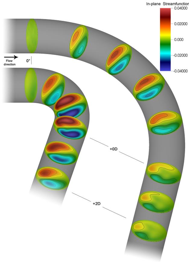
Figure 2: Formation of Dean vortices in the spatially developing  $90^\circ$  bent pipe, visualised by in-plane streamfunction ( $Re_b = U_b D / \nu = 11700$ ) (Left)  $\delta = 0.3$ , (right)  $\delta = 0.1$ . Taken from Ref. [5].
