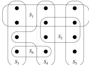
To the left is a set-covering instance  $(X, \mathcal{F})$ , where  $X$  consists of the 12 black points and  $\mathcal{F} = \{S_1, S_2, S_3, S_4, S_5, S_6\}$ . A minimum-size set cover is  $\mathcal{C} = \{S_3, S_4, S_5\}$ , with size 3.
