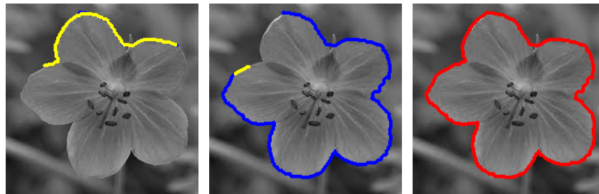
(a) Shortest path between (b) A selected/fixed curve (c) An auto-closed curve. a control point and the segment. moving mouse pointer.
