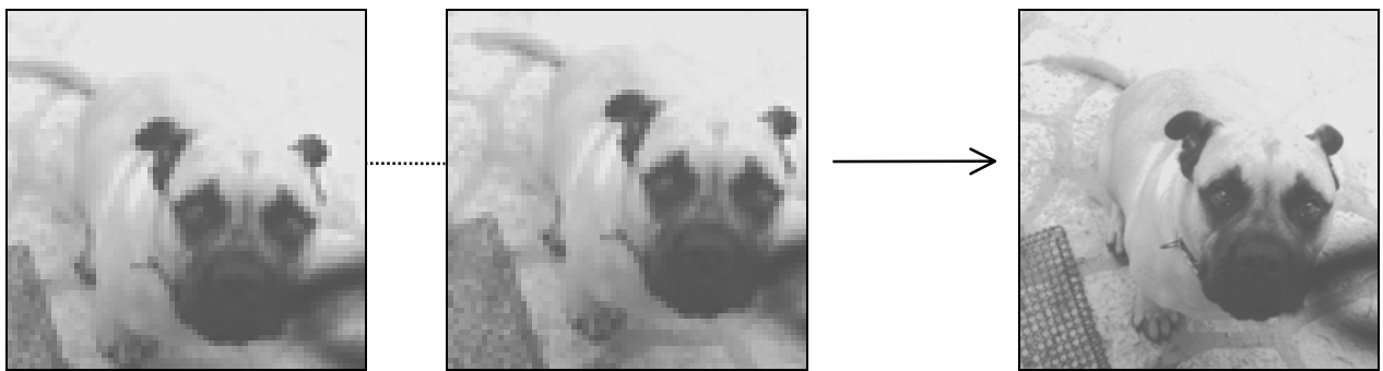
Figure 1: From a sequence of randomly shifted, undersampled images one can obtain a higher resolution image. Ideally, the algorithm should reveal the structure of the aliased object on the bottom left of the image.
