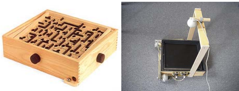
Figure 1 A Brio labyrinth, and a modified version with a camera and motors added
