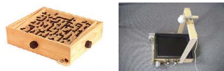
Figure 1. The Brio labyrinth, in the original version and a modified version with a camera and step-motors added
