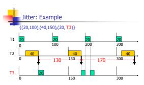
T3 is activated by T2 when it finishes within each period Note that because the response time for T2 is not a constant, the period between two instances of T3 is not a constant: 170, 130
