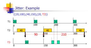
T3 is activated by T2 at any time during its execution of an instance J(biggest)= R2(worst case), J(smallest)= R2(best case)-C2 Jitter = J(biggest)- J(smallest)=60-0=60
