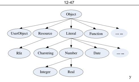
Figure 6 Part of the Amos II Built-in Types Hierarchy Chart
