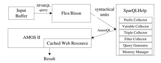
Figure 10 Architecture of SparQL Parser
