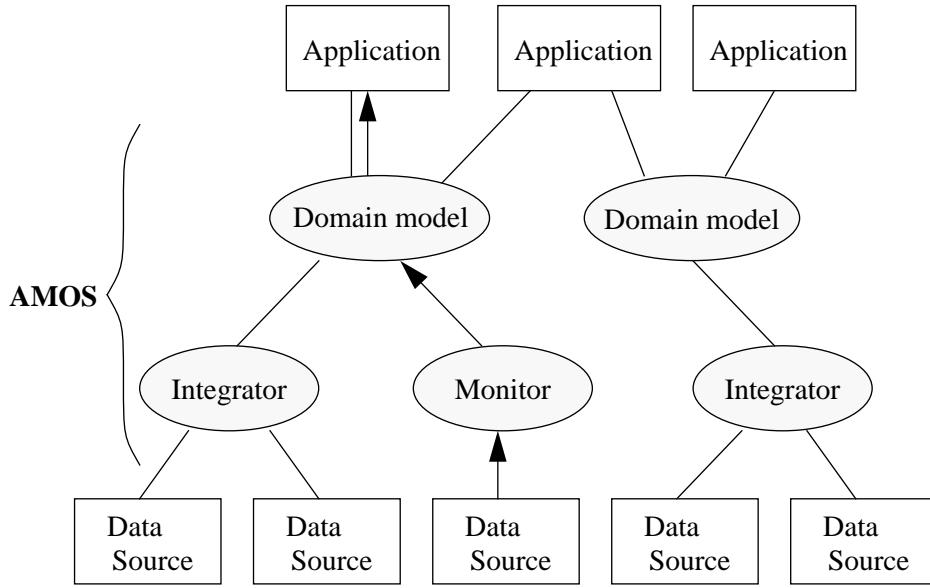
*Figure 1* Active mediators of different classes mediating between data sources and users/applications
