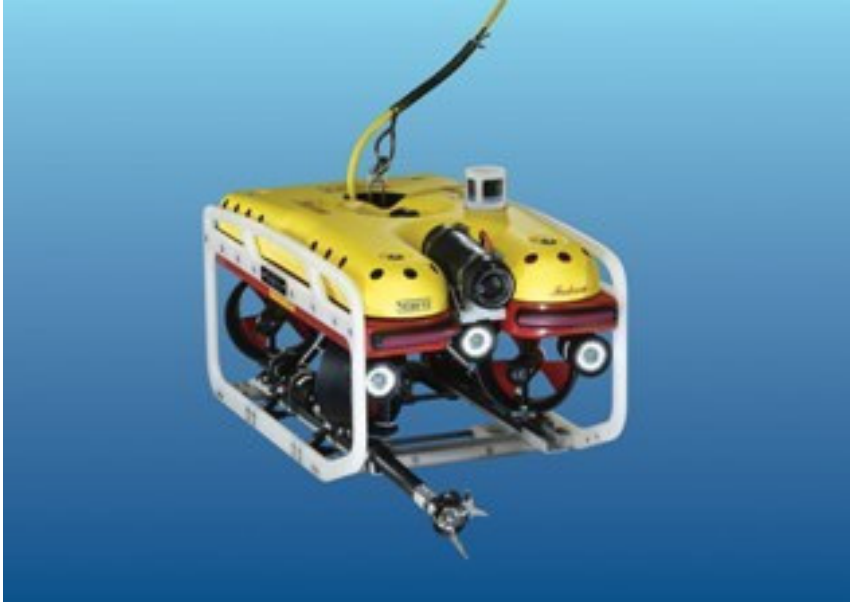
Figure 1: The Saab Seaeye Falcon vehicle that was used that was used in the experiments.
