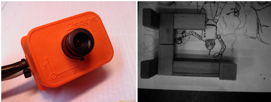
(a) The combined strap-down IMU and camera system.
