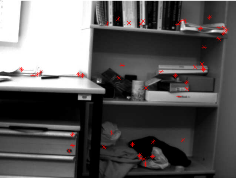
Figure 11: Example image from the free-hand run with extracted features shown as red stars.
