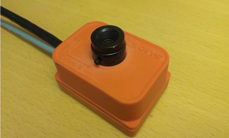
Figure 4: Sensor unit containing both camera and inertial sensors.
