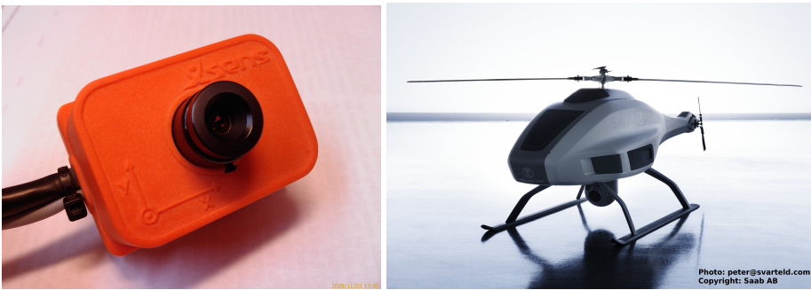
Figure 1.2: Left: Combined camera and inertial sensors in a single unit. Prototype made by XSens. Right: The Saab V-200 Skeldar helicopter. By courtesy of Saab AB.
