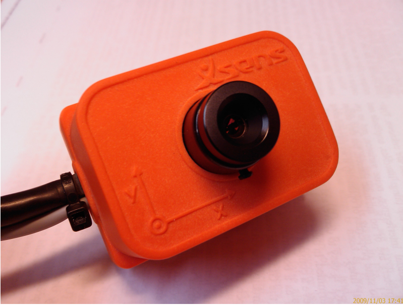
Figure 3: Sensor unit containing both camera and inertial sensors.
