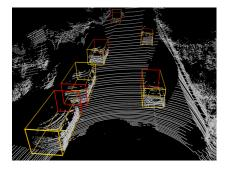
**Task:** Detect objects from sensor data (here laser), estimate their size and position in the 3D world.
