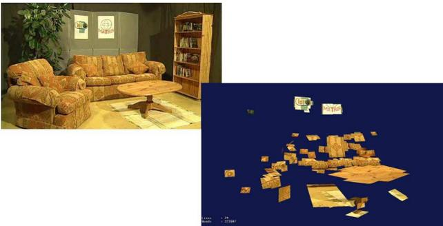
**Fig. 2** An example of a scene model consisting of planar patches (*lower right*) and the actual scene that is modelled (*upper left*).
