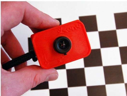
Fig. 1: The sensor unit, consisting of an IMU and a camera. The camera calibration (checkerboard) pattern is visible in the background.
