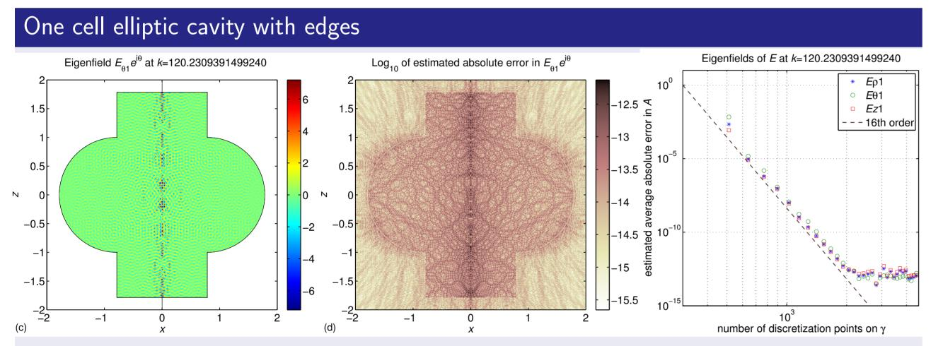
Left: The azimuthal component of normalized electric field for the 9928th n = 1eigenmode with eigenwavenumber k = 120.2309391499240 evaluated at  $4.9 \cdot 10^5$ points on a cartesian grid. Object diameter  $\approx 75\lambda$ . Center:  $\log_{10}$  of estimated absolute pointwise error. Right: stable 16th-order convergence with mesh refinement.
