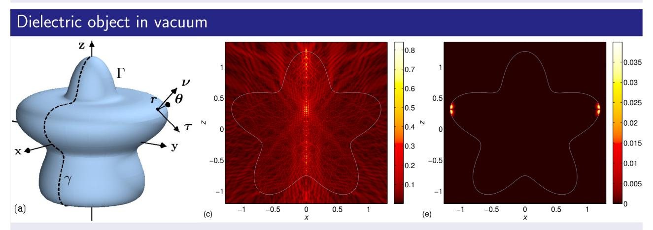
Left: Object. Center: Azimuthal component of electric field for the n = 1 eigenmode with eigenwavenumber k = 110.041232211051 - 0.404177078290i. The refractive index is m = 1.5. The object diameter is around 46 vacuum wavelengths. Right: Whispering gallery n = 450 mode with eigenwavenumber
