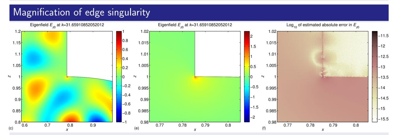
Left and center: zoom of z-component of normalized electric field for the 662nd n = 0 eigenmode with eigenwavenumber k = 31.65910852052012. The field diverges in the reentrant corners. Right:  $\log_{10}$  of estimated absolute pointwise error.
