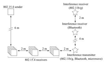
Figure 1: Experimental setup in the anechoic chamber
