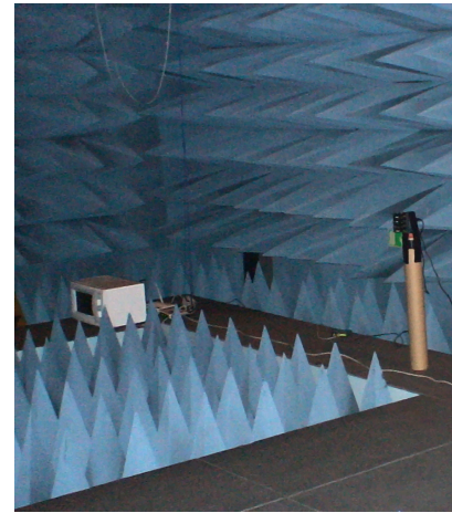
Figure 3: The microwave interferer and four of the sensor nodes (on a tripod) in the anechoic chamber
