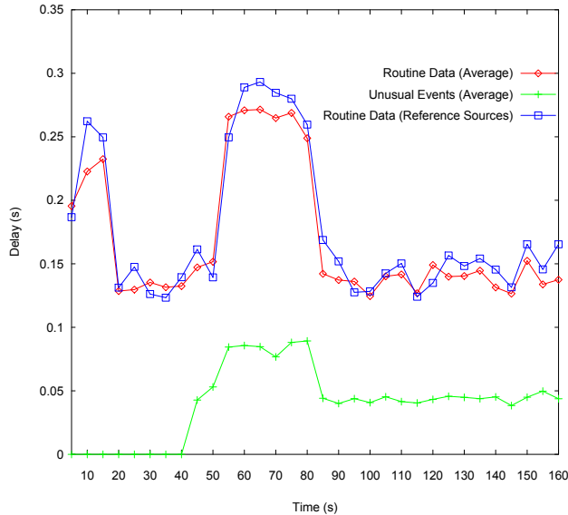
Fig. 6. Unusual events achieves lower packet travel delay after RRR is applied at 40s, while the delay of routine data increases as they are spread aside to some secondary paths. At 80s, traffic reduction is adopted by dropping the routine data packets with probability p_d = 0.1 to reduce the network traffic and the packet delay.
