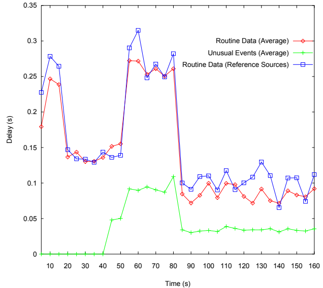
Fig. 7. The packet travel delay is further reduced when the dropping probability increases to p_d = 0.2 .
