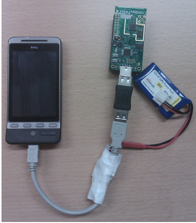
Fig. 9. Attaching a Tmote Sky sensor to a HTC Hero smart phone.
