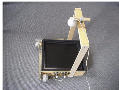
Figure 1. A Brio labyrinth, and a modified version with a camera and motors added (from Berglund, 2002). The aim of the game is to move a steel ball on the board from a starting point to a final point. The knobs are used to tilt the board and in this way move the ball
