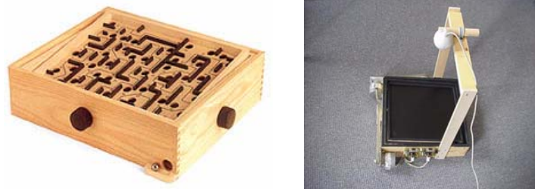
Figure 2. A Brio labyrinth and a modified version with a camera and motors added (from Berglund, 2002a). The aim of the game is to move a steel ball on the board from a starting point to a final point. The knobs are used to tilt the board and in this way move the ball
