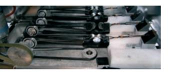
The test setup in the solar radiation chamber. The antenna arms are folded to reduce the size of the setup. On the left side is the motor to induce vibrations.
