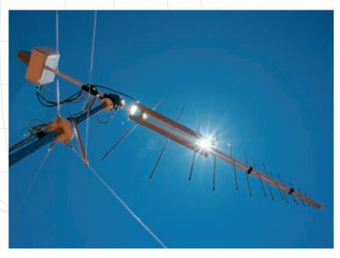
Some of the ASTRON monitoring equipment, mounted in a 5 metre tall mast. To the right a low frequency antenna and to the left a frontend with the sensitive receiver electronics inside and an integrated high frequency antenna in a radome.
