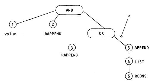
(REMREC can remove recursion under "chains" of function calls in the last argument to append, list, cons, nconc, rplaca and rplacd. In the example we have a "chain" of append and list)
