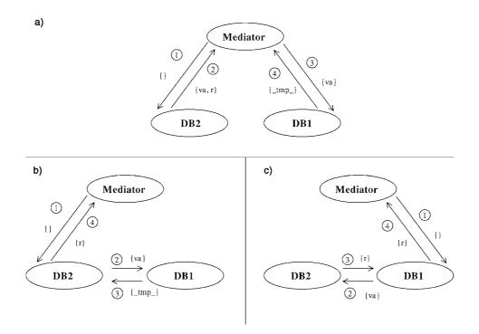
Figure 11. Execution diagrams of the decomposition tree of the example query before node merge and after.
