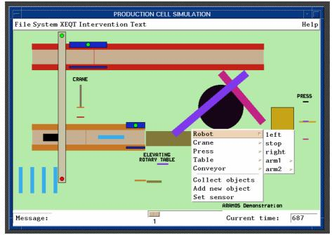
Fig. 3. A top-view of a simulated production cell for manufacturing car body parts
