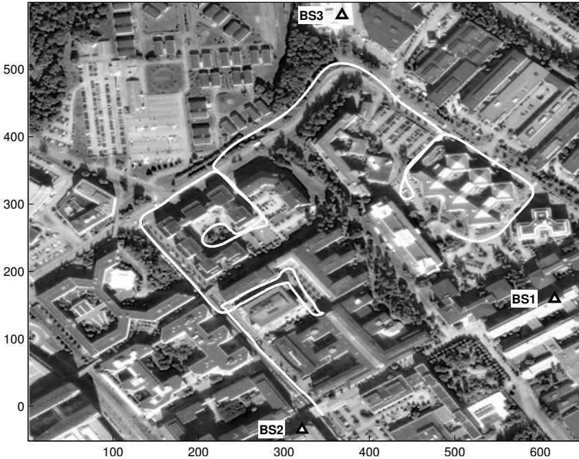
Figure 3: Configurations of the three base stations used in the experiment in Kista, Stockholm. The driven trajectory is in white starting near base station 2 in the lower part of the image.
