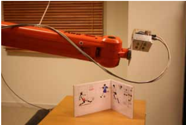
Figure 6.5: A prototype of the sensor unit is mounted onto an industrial robot. The background shows the scene that has been used in the experiments.
