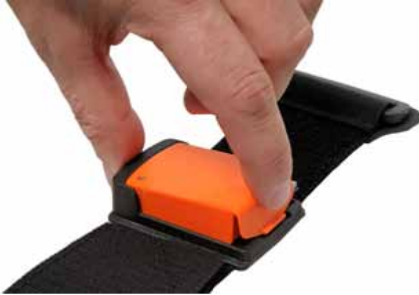
Figure 5.1: An Xsens MTw, a wireless IMU, is placed in an easy-to-wear strap.
