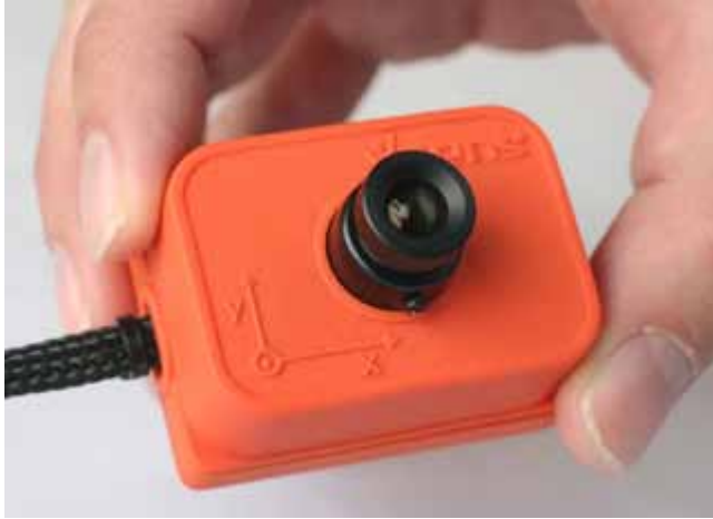
Figure 6.2: An Xsens prototype sensor unit, integrating an IMU and a camera into a single housing.
